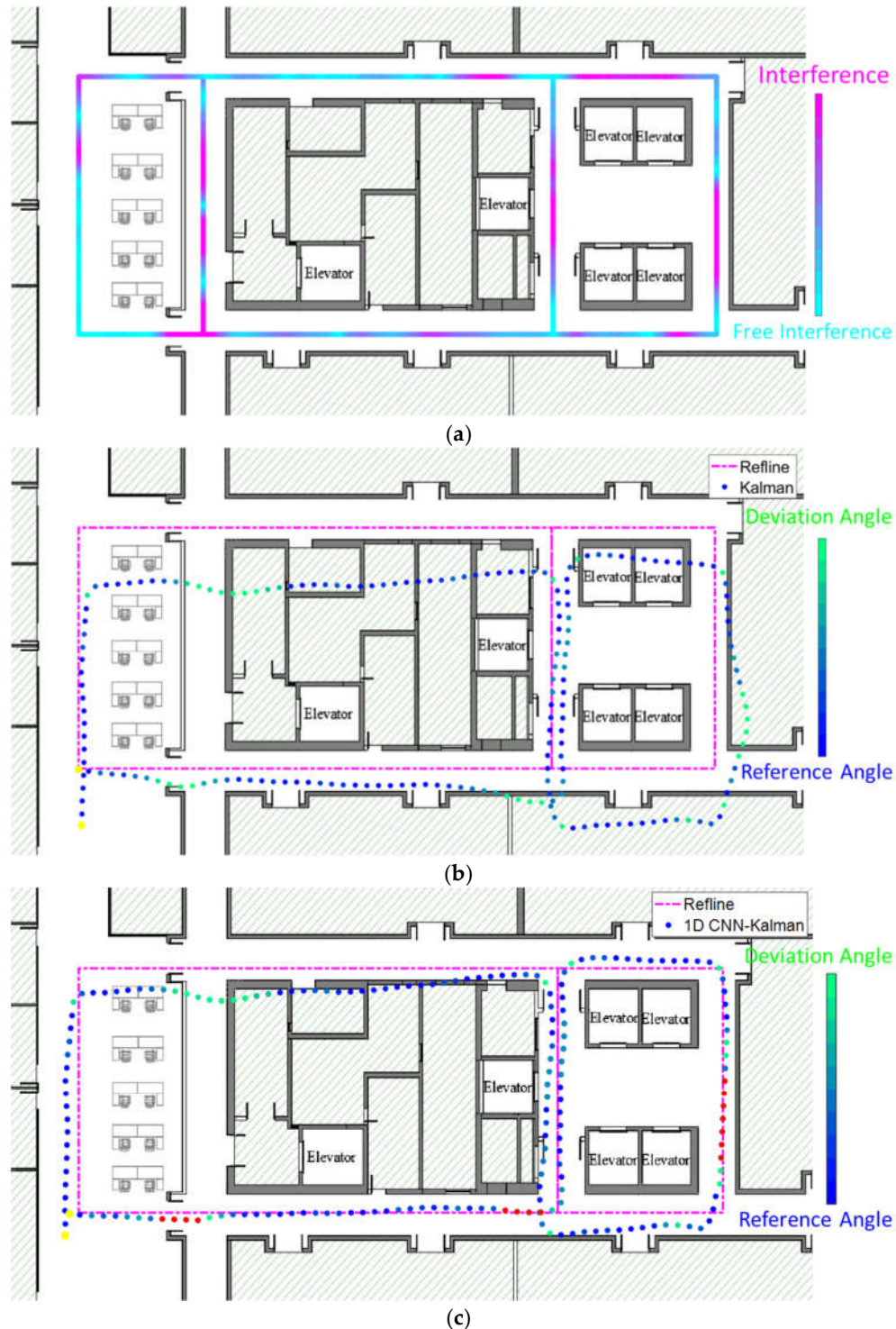
Figure 6. (a) The measurement of magnetic field in an indoor environment. (b) The distribution of heading angle based on Kalman. (c) The distribution of heading angle based on 1D CNN–Kalman.
