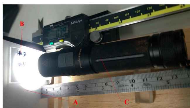
Figure 11. Focal length measurement of the microlens, where A is the screen, B is the microlenses, and C is the light respectively.
