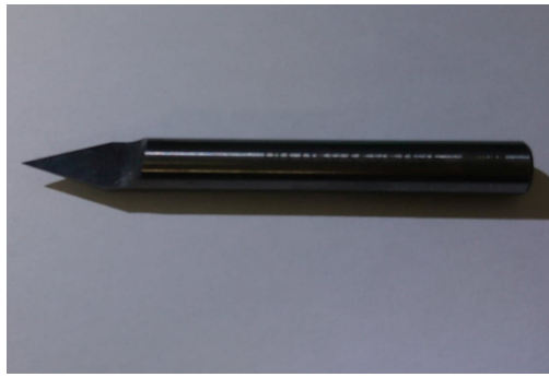
Figure 1. Tungsten steel microshaper. The microshaper is mounted on a CNC machine to machine the microlens.
