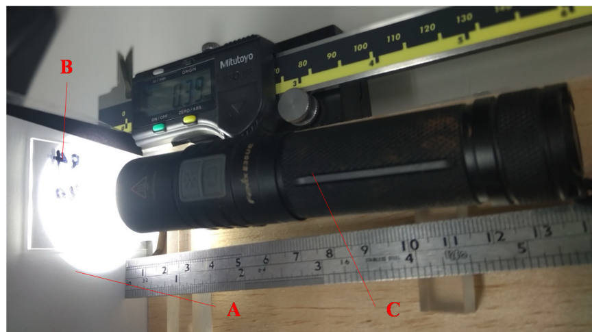
Figure 11. Focal length measurement of the microlens, where A is the screen, B is the microlens, and C is the light respectively.
