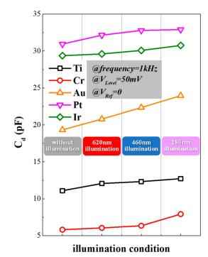
**Figure 6.** The change of  $C_d$  versus the wavelength ( $V_{Ref} = 0$  and  $V_{Level} = 50$  mV at 1 kHz) of microelectrodes caused by different surface materials.
