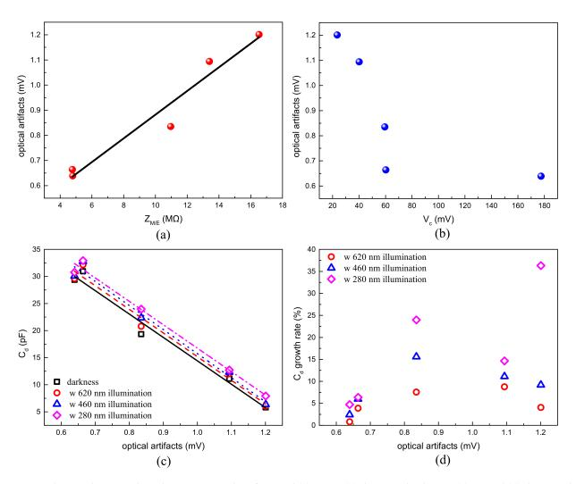
**Figure 8.** The correlation analyses between optical artifacts and (a)  $Z_{M/E'}$  (b) the critical value  $V_c$ , (c)  $C_d$  and (d) the growth rate of  $C_d$ , respectively.
