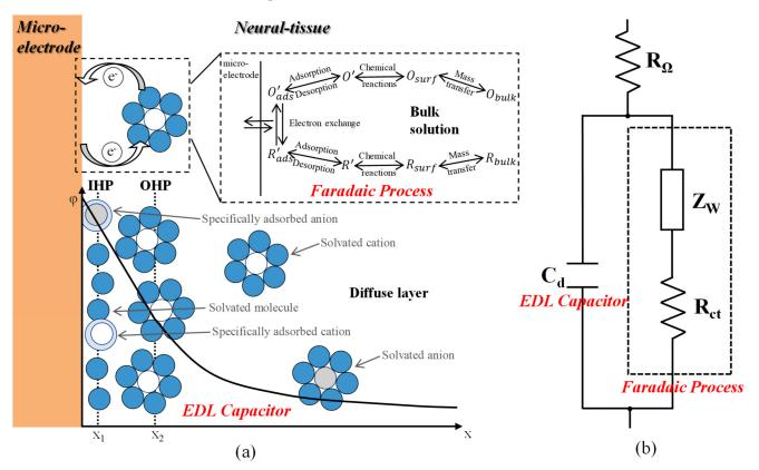
**Figure 2.** (**a**) Theoretical model for the charge transfer mechanism on the microelectrode/electrolyte interface, in which the upper part displays faradaic processes and the lower part an EDL capacitor. (**b**) Equivalent circuit for the charge transfer mechanism on the interface.
