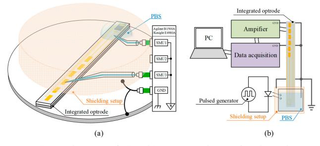
**Figure 3.** (a) The proposed testing system for electrical characterizations with a semiconductor device analyzer or LCR meter in PBS with shielding. (b) The testing system for optical artifacts with amplifier and data acquisition card in PBS with shielding, while the optical artifacts are generated by a light-emitting diode driven by a pulse generator.
