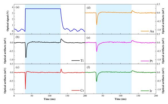
**Figure 7.** (a) The optical signal used in the testing system and the recorded optical artifacts of optrodes made by different surface materials, including (b) Ti, (c) Cr, (d) Au, (e) Pt, (f) Ir.
