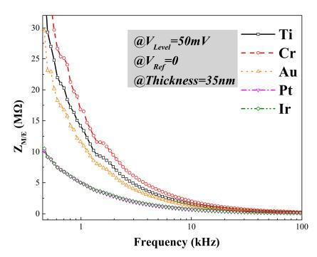
**Figure 4.** Electrochemical impedance spectroscopy (EIS) of microelectrodes with different surface materials, including Ti, Cr, Au, Pt and Ir.
