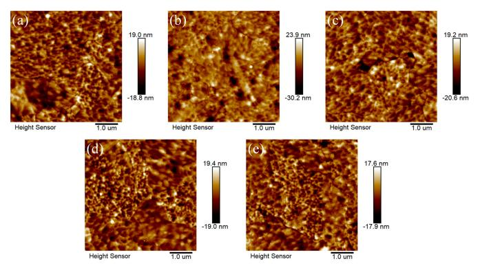
**Figure A1.** 5  $\mu$ m × 5  $\mu$ m AFM images of microelectrodes made of (a) Ti, (b) Cr, (c) Au, (d) Pt, (e) Ir.
