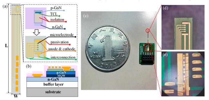
(MOCVD) system, comprising a GaN buffer layer, an *n*-GaN layer, GaN/InGaN MQWs, an AlGaN electron blocking layer and a *p*-GaN layer, from the bottom to the top.
