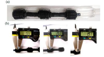
**Figure 4.** Soft robotic finger: (**a**) a fabricated soft robotic finger with three multi-material pneumatic actuators; (**b**) different size of each pneumatic actuator.
