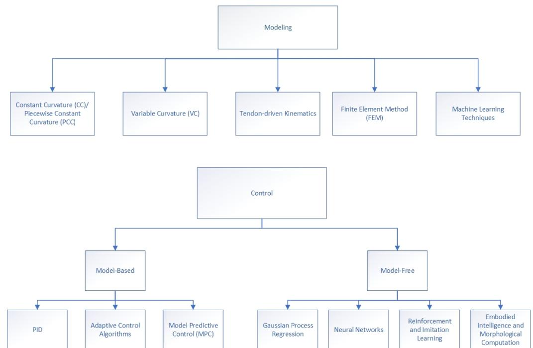
**Figure 2.** An overview of the different modeling and control techniques used in soft robotics.
