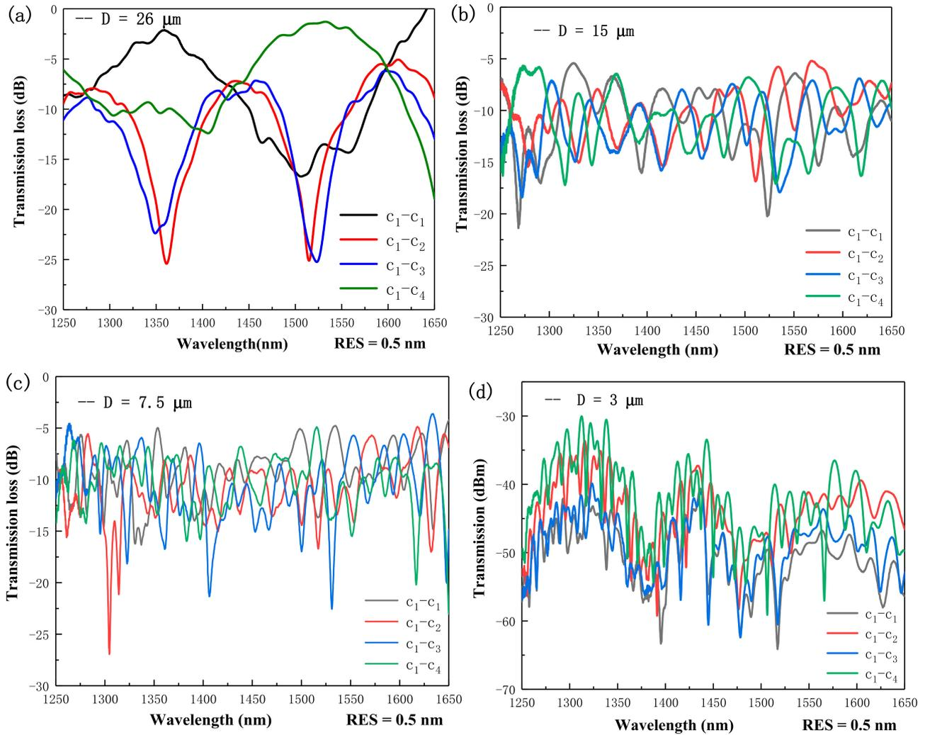
**Figure 2.** Spectral responses of the oscillating curves for (a)  $D = 26 \mu\text{m}$ , (b)  $D = 15 \mu\text{m}$ , (c)  $D = 7.5 \mu\text{m}$ , and (d)  $D = 3 \mu\text{m}$ , for the  $c_1-c_{1/2/3/4}$  coupling states.
