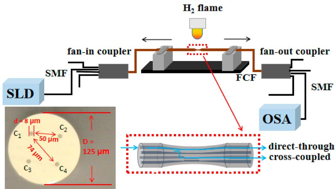
**Figure 1.** Experimental set-up of the tapered FCF interferometer in which  $c_1$ ,  $c_2$ ,  $c_3$ ,  $c_4$  represent the excitation core, two neighboring cores, and diagonal cores, respectively. The inset picture shows the designation of the four cores of the un-tapered FCF under  $1000\times$  CCD microscope.
