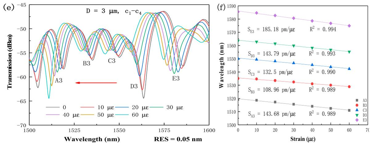
**Figure 3.** Spectral responses of the TFCF interferometer under different tensile strain for (a)  $D = 15 \mu\text{m}$ , (c)  $D = 7.5 \mu\text{m}$ , and (e)  $D = 3 \mu\text{m}$ , respectively. Linear fitting curves of the dip wavelength shifts and the coefficients of determination  $R^2$  of linear fitting for (b)  $D = 15 \mu\text{m}$ , (d)  $D = 7.5 \mu\text{m}$ , and (f)  $D = 3 \mu\text{m}$ , respectively.
