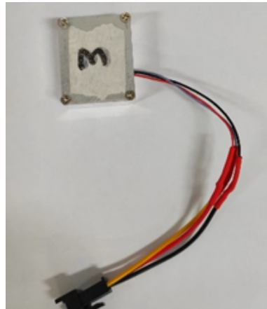
Figure 5. The overall packaging of the accelerometer.
