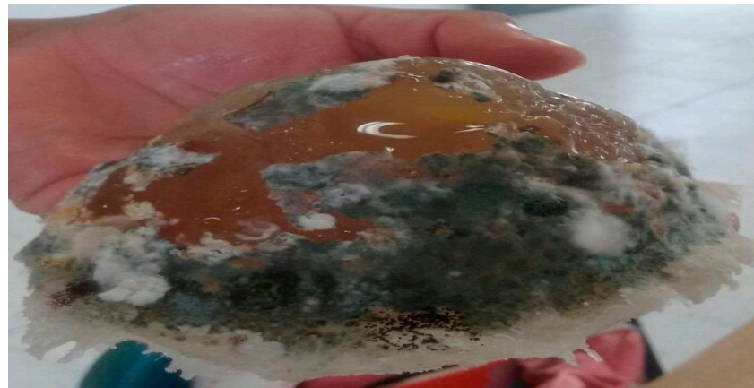
Figure 2. Decomposition of the normal tissue phantom after 2 months.
