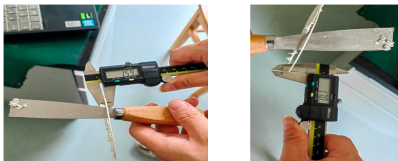
Figure 20. Measurement of the thickness of a printed single-layer circle.
