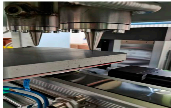
Figure 19. Experiment of extruding PBX into threads.
