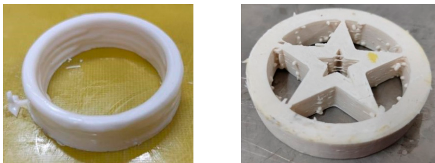
Figure 23. Hollow circle structure modeling and printed sample.
