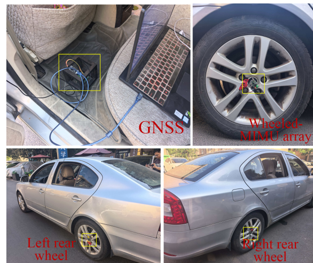
Figure 3. Installation of the wheeled MIMU array for vehicle experiments.
