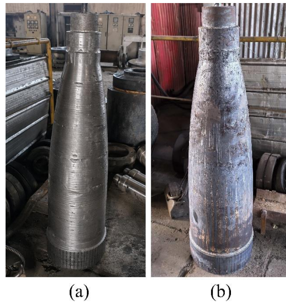
Figure 11. Macroscopic forming morphologies of hot-spun workpieces under different temperature conditions: (a) 750 K and (b) 1200 K.
