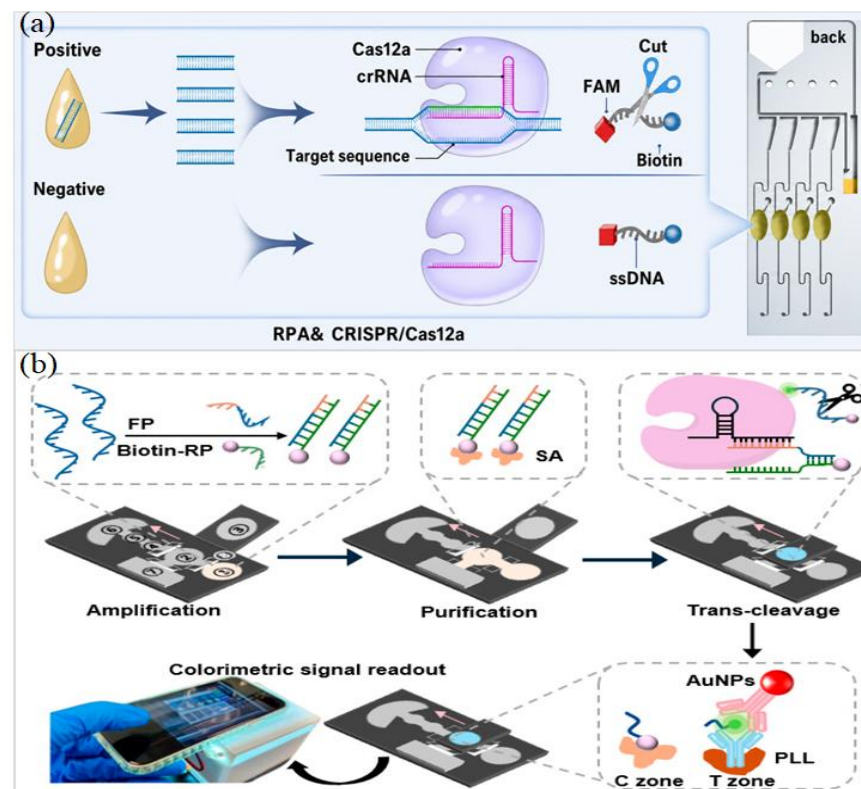
Figure 1. (a) Schematic illustration of a CRISPR-assisted microfluidic RPA chip for the detection of multiple respiratory viruses. (Reprinted from Ref. [59]). (b) Schematic representation of a \mu PAD-based platform integrating RPA and colorimetric CRISPR/Cas12a for HPV16 E7 detection. (Reprinted from [36]).
