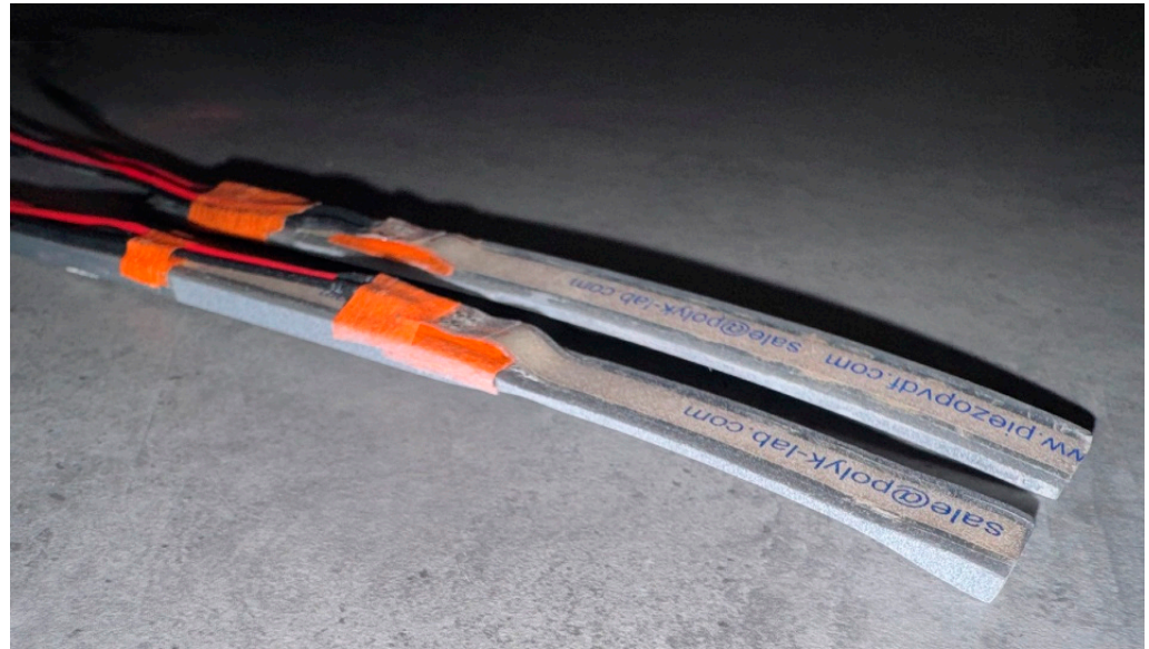
Figure 13. Illustration of the manufactured cantilevers—top cantilever is uniform thickness shape, and bottom cantilever is optimal shape.
