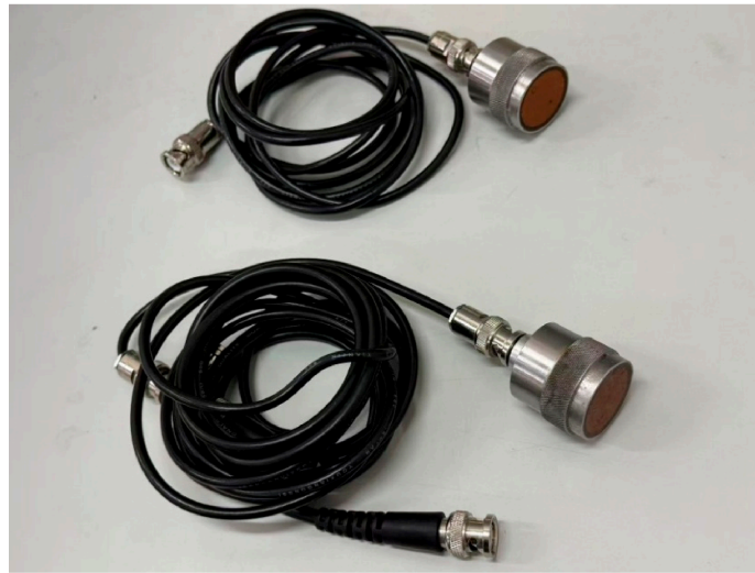
Figure 6. Physical images of the source and receiving transducers.
