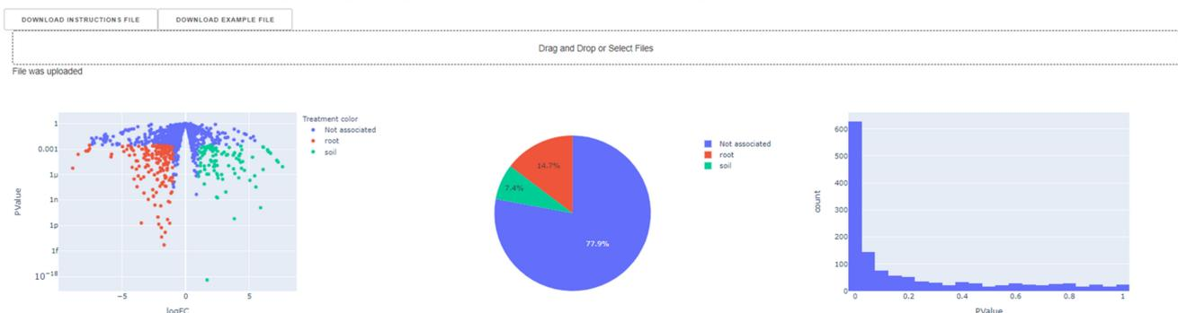
**Figure 1.** User interface of NetCom following the upload of the input file. Input files are uploaded via the 'Drag and Drop or Select File' bottom. An example input file is available (via the 'Download example file' grey bottom, top left). Once a valid file is introduced, the three plots on the bottom are generated.
