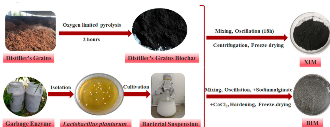
Figure 1. Flow charts of ordinary distiller's grains biochar, XIM, and BIM preparation.
