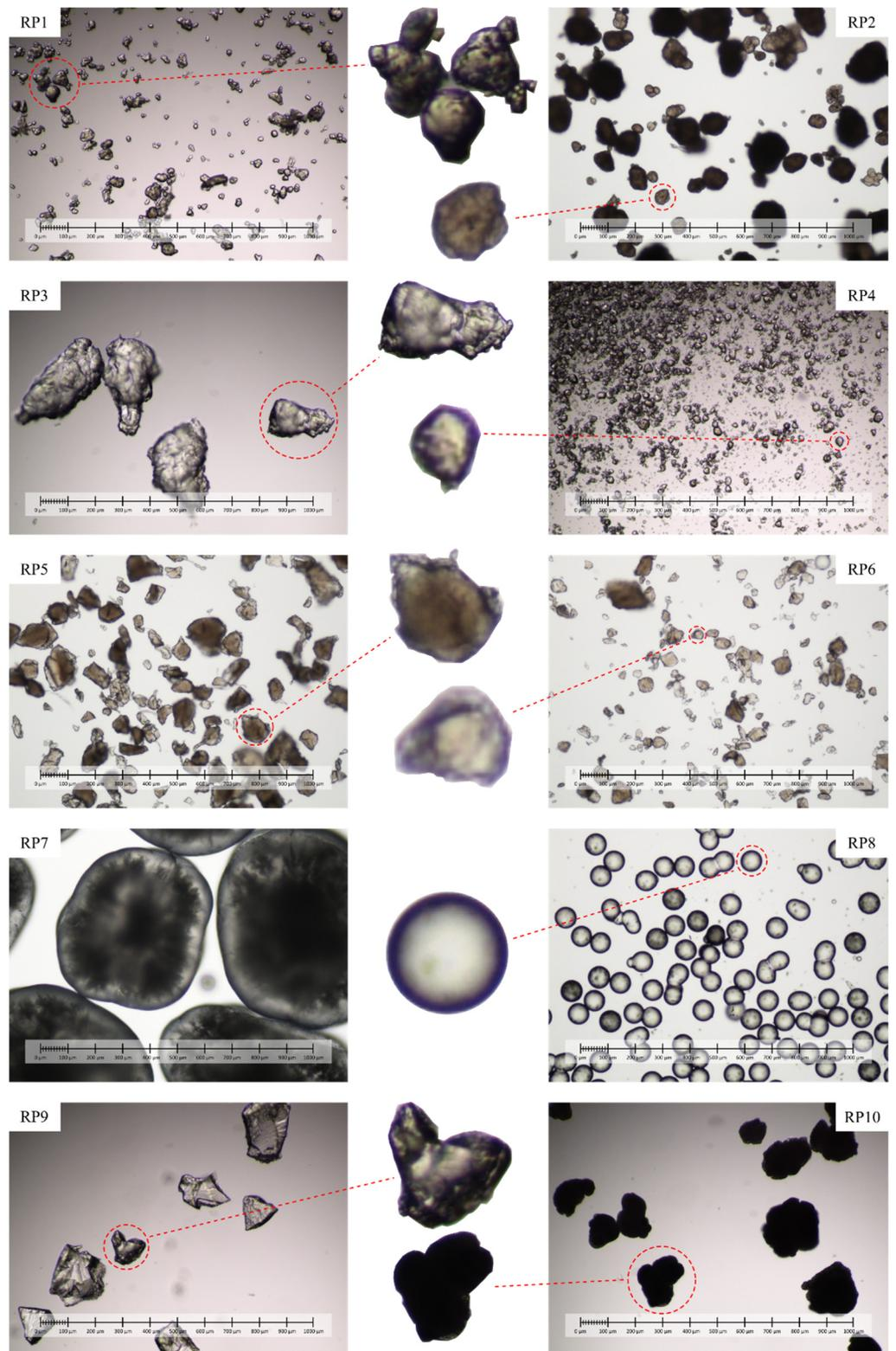
**Figure 2.** Microscope photos for evaluation of particle shape of reference particles RP1–RP10. The scale shown indicates the particle size from 0–1000 μm.
