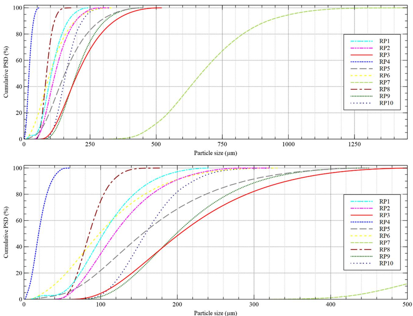
**Figure 1.** Particle size distribution (PSD; cumulative) of the microplastic particles for comparison. The upper figure describes the distribution sum over the entire measuring range up to 1450  $\mu\text{m}$ . The lower figure shows a magnification for the particle size range up to 500  $\mu\text{m}$ .
