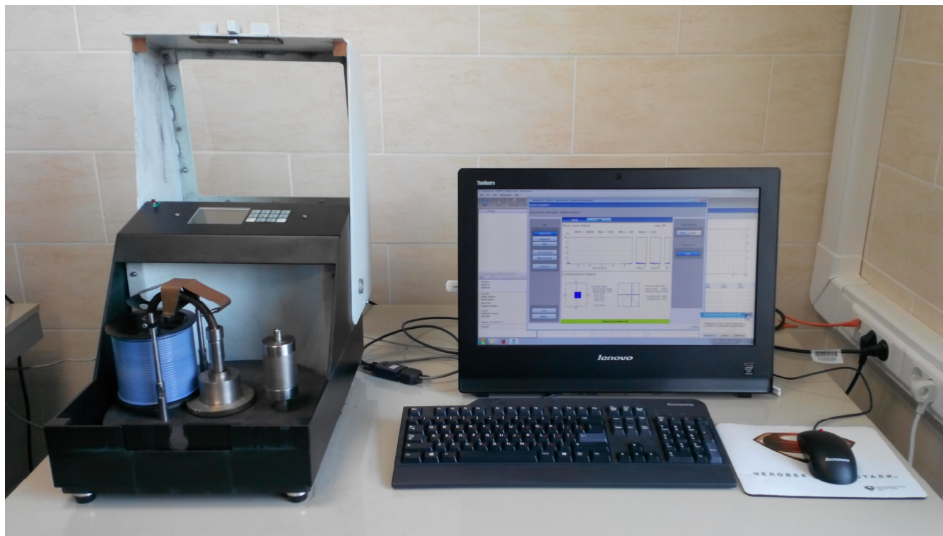
Figure 2. Planetary centrifuge with a vertical single-layer rotating coiled column.
