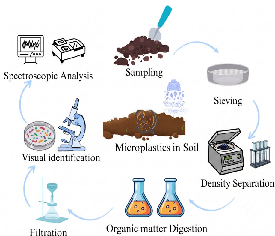
Figure 3. Typical workflow for microplastic extraction and analysis from soil samples, from sample collection through density separation, organic matter digestion, filtration, and microscopic examination.
