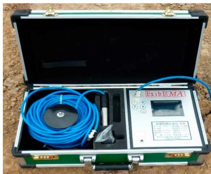
Figure 5. TYGD10 stratum borehole monitor.
