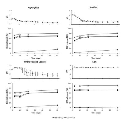
**Figure 2.** Changes in pH (top section of graphs) and release of La, Dy, Lu and Ce (bottom sections of graphs) over the duration of the experiment. Day zero pH measurement was taken 1 h after mixing IAD. The chemical analysis starts from day three as first data point. Error bars are standard deviation of triplicate measurements.
