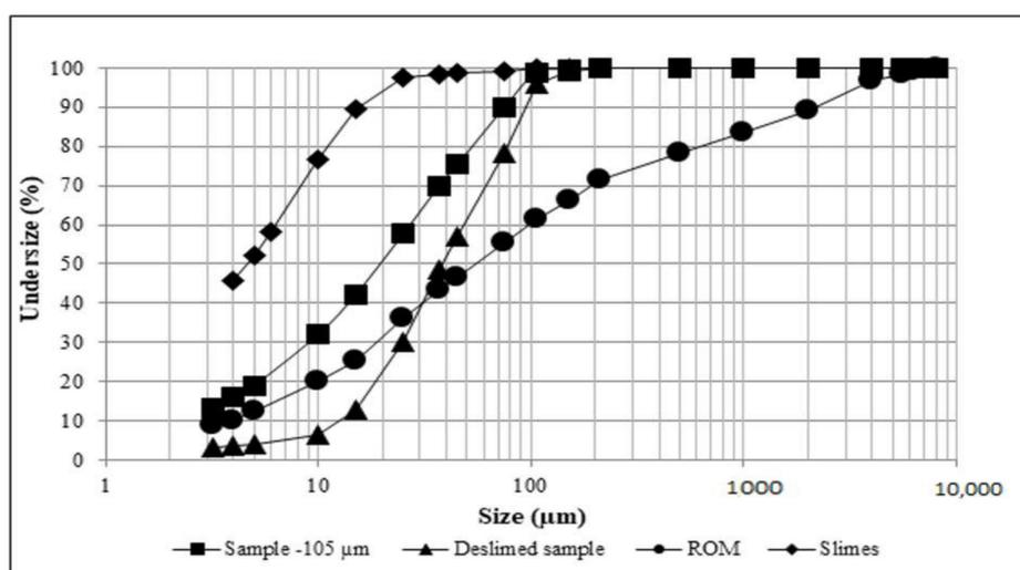
**Figure 2.** Size distribution curves of the amphibolitic itabirite samples studied: run of mine (ROM),  $-105 \mu\text{m}$ , deslimed and slimes.
