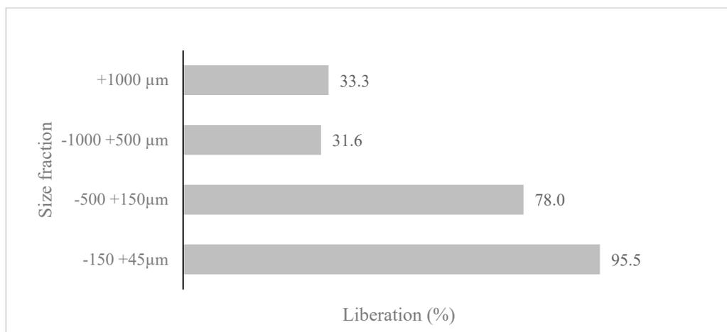
**Figure 7.** Quartz liberation in regard to the iron minerals of amphibolitic itabirite.
