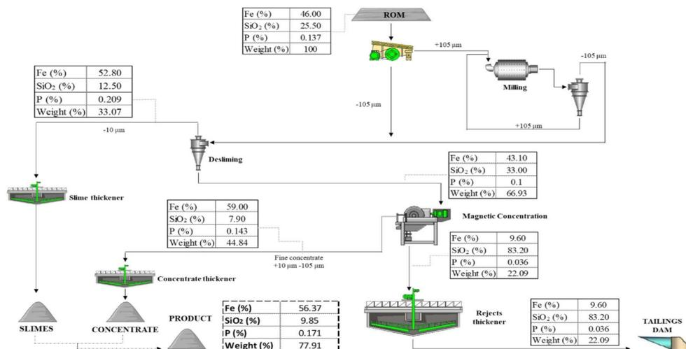
**Figure 8.** Proposed flowsheet of the magnetic concentration of the amphibolitic itabirite (open circuit).
