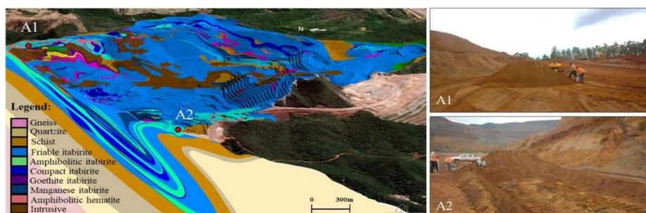
**Figure 1.** Geological section and map of Brucutu's deposit, with the location of the two regions where the subsamples A1 and A2 (right side) of the amphibolitic itabirite were collected.
