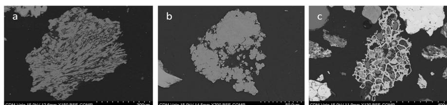
**Figure 6.** Backscattered electron images of the SEM, showing microtextures of goethite from the studied amphibolitic itabirite: (a) fibrous amphibolitic, (b) massive and (c) alveolar.
