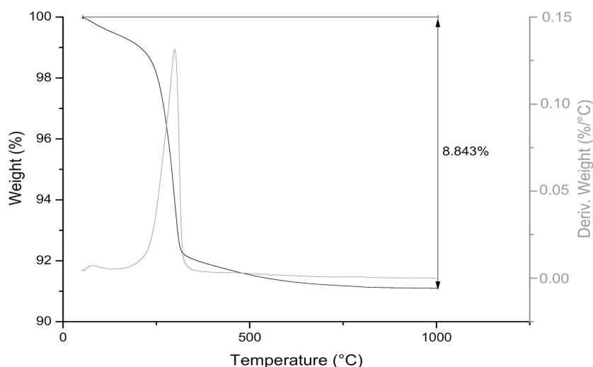
**Figure 4.** Thermogram of the size fraction  $-45\ \mu\text{m}$  of the amphibolitic itabirite (ROM).
