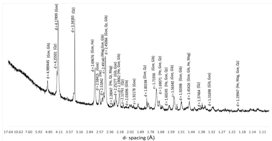
**Figure 3.** X-ray diffraction pattern of the size fraction  $-45\ \mu\text{m}$  of the amphibolitic itabirite (ROM).
