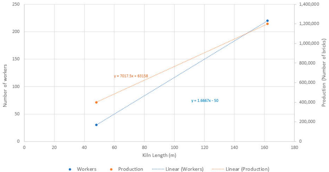
**Figure 10.** Relationship between kiln length (m) observed in satellite imagery and the per kiln work force and production values published in [7].
