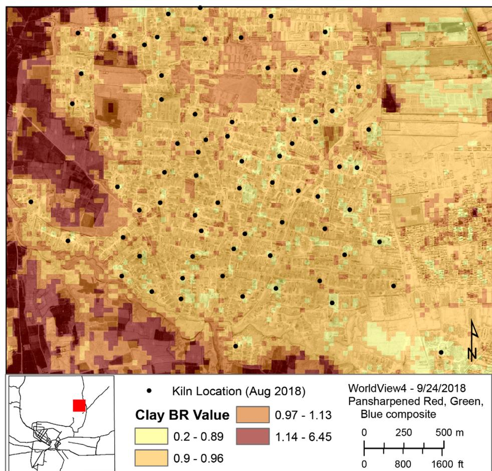
**Figure 13.** Area of detail showing the result of the clay band ratio analysis, overlain by kiln locations (black points).
