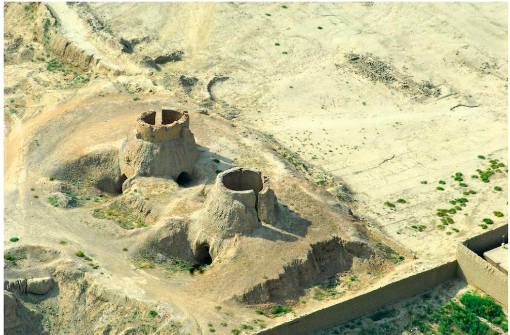
**Figure 4.** Inactive artisanal clamp-style brick kiln, photographed on 8 July 2012 in Kabul, Afghanistan. Photograph by: ajax, licensed under CC BY 3.0.
