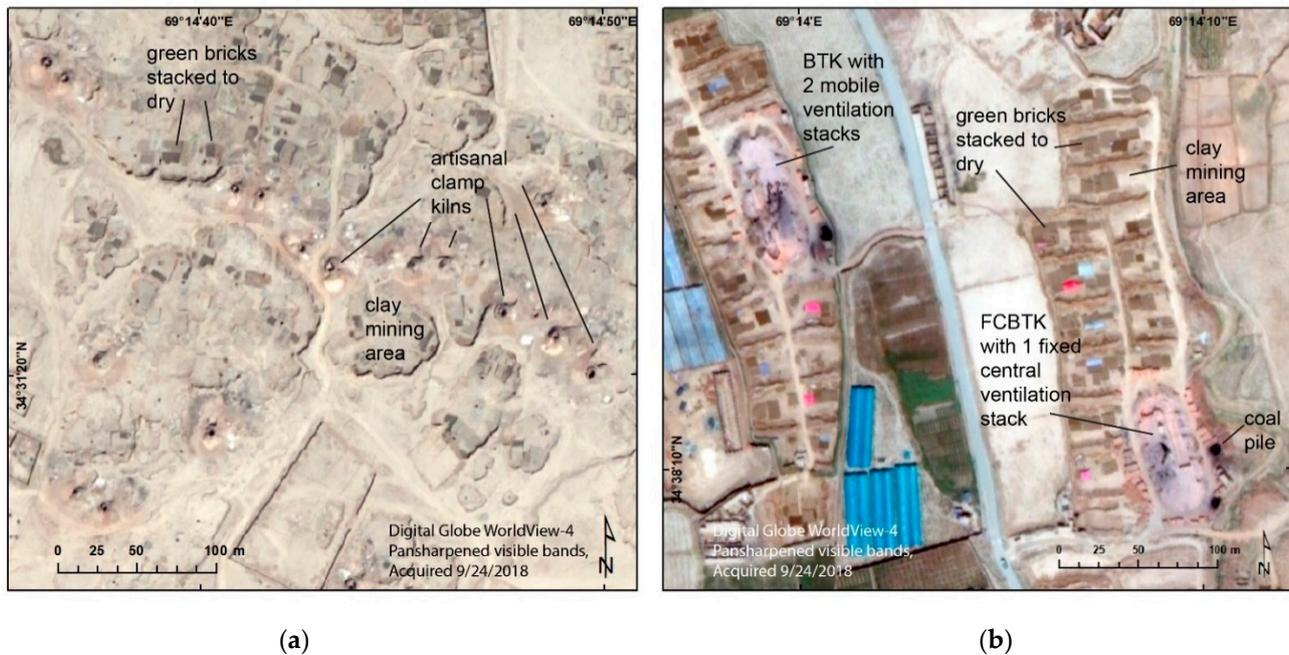
**Figure 7.** Examples of the kiln types found in the study area: (a) clamp kilns; (b) Bull’s Trench Kiln (BTK) with 2 mobile ventilation stacks and Fixed Chimney Bull’s Trench Kiln (FCBTK).
