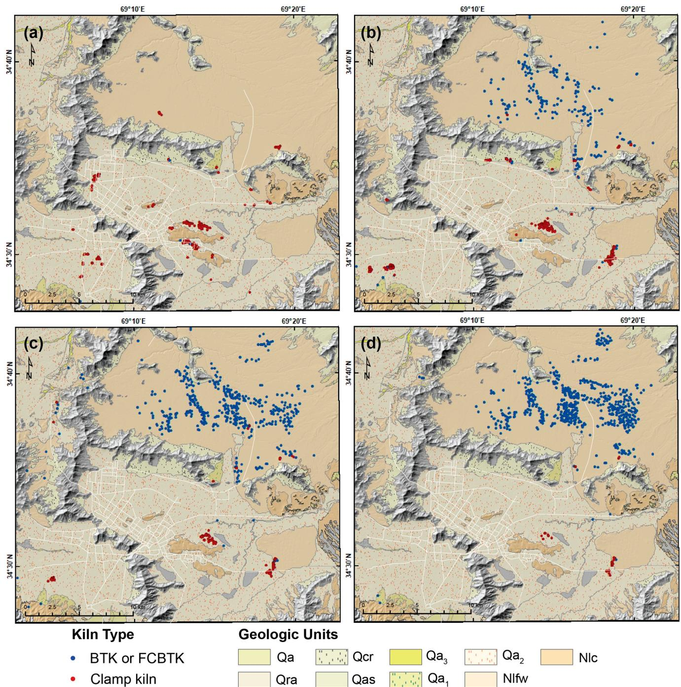
**Figure 9.** Kiln locations in the Kabul region, mapped by date and type (Clamp kiln, BTK, or FCBTk) and overlain on surficial geology adopted from [18]. (a) 1965; (b) 2004; (c) 2011; (d) 2018.
