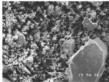
**Figure 3.** Microstructure images of copper slag at 330 $\times$  magnification and 50  $\mu\text{m}$  scale.
