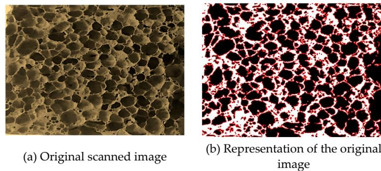
**Figure 7.** Digital processing of the scanned geopolymer foam plates. (a) Original scanned image of the saw-cut flat surface of a sample; (b) with black representing the voids, white the flat material matrix and red the extracted void boundaries.
