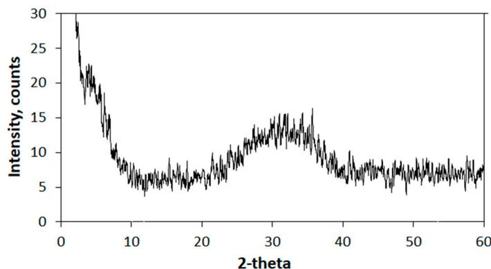
**Figure 2.** XRD pattern of copper slag.
