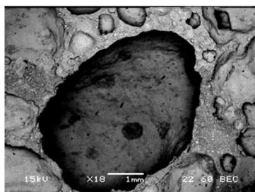
**Figure 6.** Scanning electron microscopy images of GeoFoam at magnification  $\times 18$  and scale 1 mm (S/L: 3.5 g/mL, [KOH]: 8 M, Al powder addition: 15 wt.%, curing: 48 h at 70 °C).
