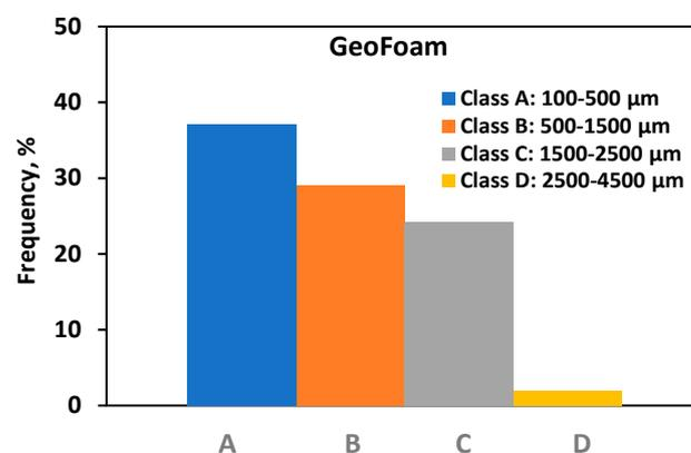
**Figure 8.** Image J analysis results for frequency % of voids/cm<sup>2</sup> (vertical axis) against the distribution of the void sizes (area—cm<sup>2</sup>) (horizontal axis) in GeoFoam sample.
