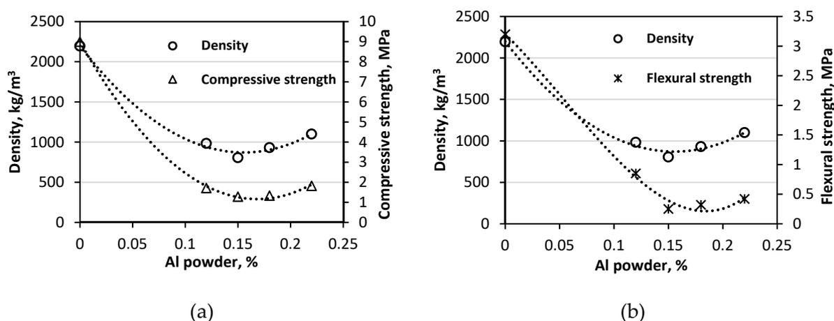
**Figure 5.** Density values and (a) compressive strength, (b) flexural strength of geopolymer pastes after 28 days of hardening, in function of different % Al powder additions at S/L: 3.5 g/mL, 8 M KOH and 70 °C curing temperature.
