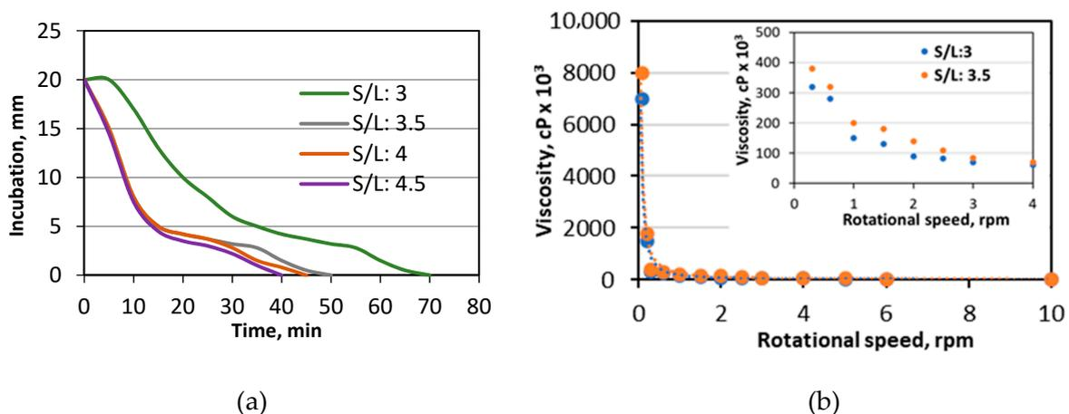
**Figure 4.** Effect of S/L ratio on the (a) setting time and (b) viscosity of geopolymer pastes with [KOH]: 8M. and curing temperature 70  $^{\circ}\text{C}$ .
