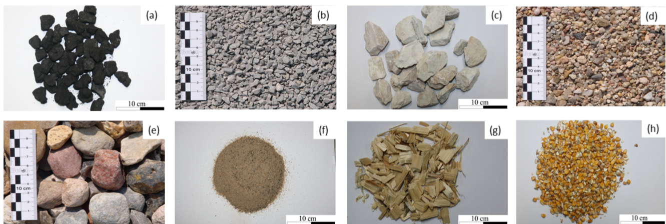
Figure 3. Granular materials considered to quantify the boundaries of the investigated material domain: (a) coke; (b) stone chippings 2–5 mm; (c) limestone; (d) gravel 2/8 mm; (e) gravel 16/32 mm; (f) dry sand; (g) woodchips; (h) dry corn.
