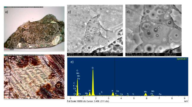
**Figure 7.** Blackening alteration: (a) OM documentation of fragment KK\_d12; (b) detail of black stains under OM ( $100 \times$ ); (c,d) BSE images of the lamellar structure, with details of concentric pits; (e) EDS spectrum acquired on the pits.
