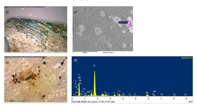
**Figure 3.** Iridescence on glass fragment KK\_d3: (a) OM documentation; (b) magnified detail of the black stains  $(100 \times)$ ; (c) BSE image of the surface; (d) EDS spectrum acquired on the black stains.
