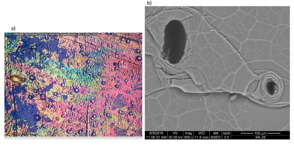
**Figure 2.** Iridescence on glass fragment KK\_d1: (a) OM documentation, highlighting the occurrence of bubbles due to the leaching progress followed by pitting; (b) BSE image of the surface, with details of the cracking network and a micrometric pore, in the white rectangle.
