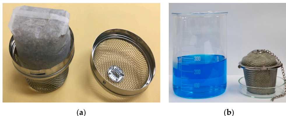
Figure 2. (a) Picture of the unlocked prototype absorbent assembly consisting of a stainless-steel mesh container and an absorbent paper pouch made of eVMTs. (b) Image of the experimental setup for a liquid mitigation test using the prototype absorbent assembly. The solution was intentionally colored by a blue dye for visibility.
