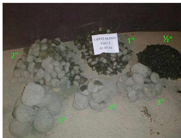
Figure 4. SAG mill internal ore charge after SAG-2 test
