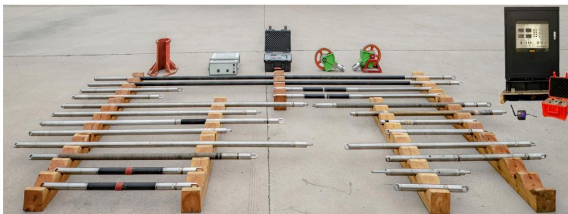
**Figure 17.** Real picture of the induced polarization logging device.
