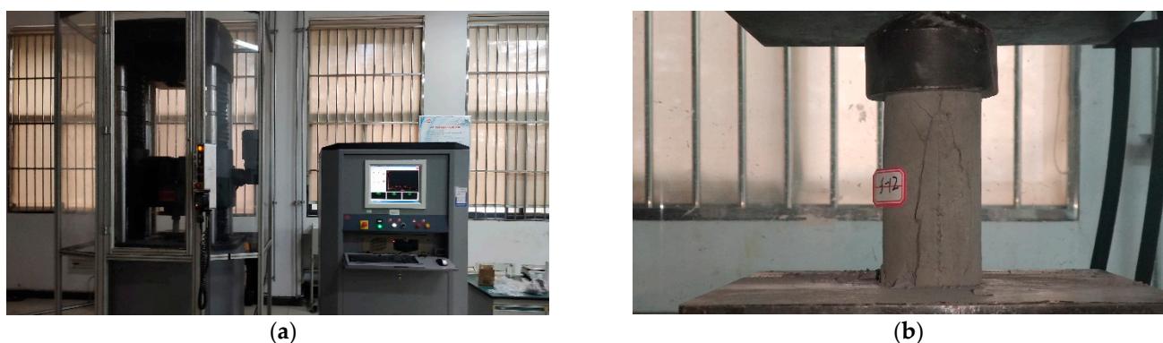
Figure 11. Loading system. (a) Experimental system, (b) uniaxial compression.
