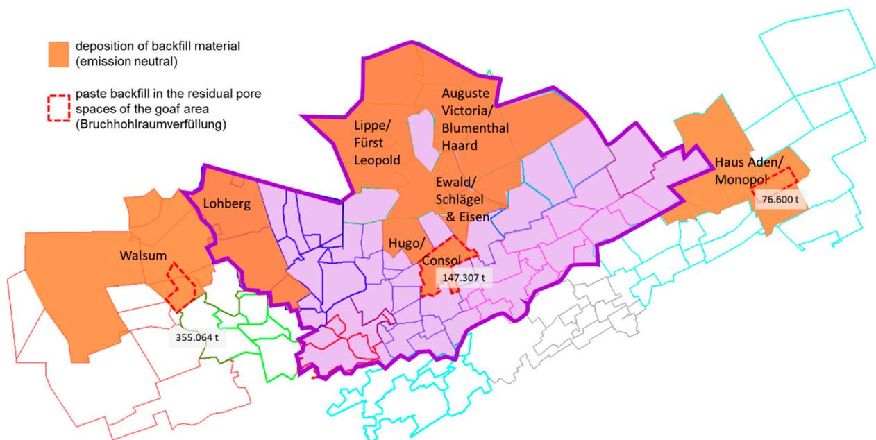
**Figure 2.** Overview on the backfill material in the Ruhr area based on [20].
