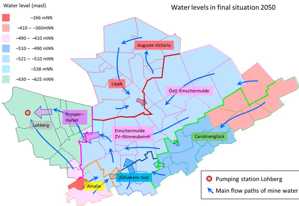
**Figure 6.** Predicted water levels and water flow directions in the Central Water Province in final situation in 2050.
