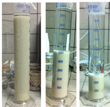
Figure 4. Time evolution of suspension height during the sedimentation test.
