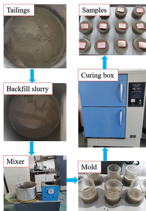
Figure 3. Preparation process of CTB specimens.
