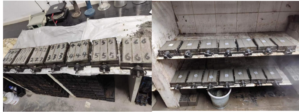
Figure 4. Molded mortar specimens.
