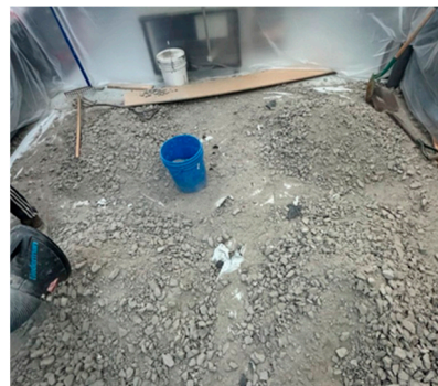
Figure 19. The waste rock supplied by Mine A and prepared for the large-scale tests using the quartering method.
