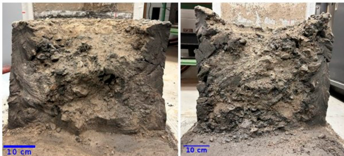
Figure 22. The internal texture structure of the large-scale test samples after sectioning through the center: Test 1 (left) and Test 2 (right).
