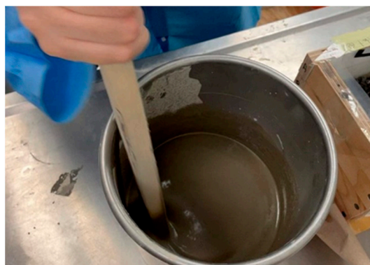
Figure 4. Manual preparation of paste backfill by mixing tailings and water.
