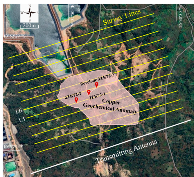
Figure 2. Satellite image and survey layout of the Ksignal area. The yellow parallel lines indicate the UAV-based semi-airborne transient electromagnetic survey lines, while the white line marks the position of the grounded transmitting antenna. Red location markers denote the boreholes used for geological control, and the shaded area outlines the projected extent of the known copper geochemical anomaly.
