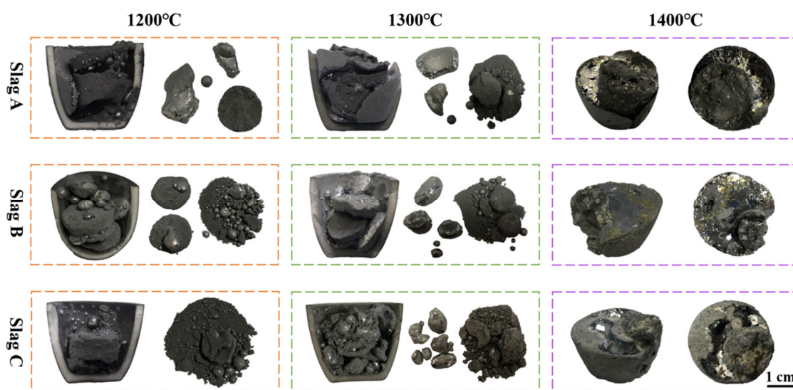
Figure 7. Macroscopic morphologies of products obtained at different smelting temperatures and CaO-Al 2 O 3 -CaF 2 slag compositions.
