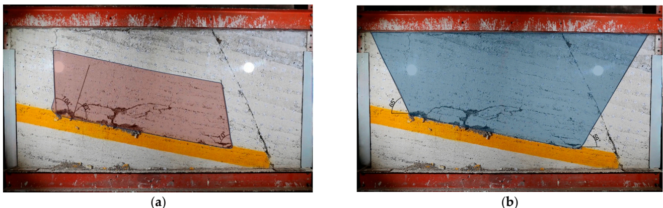
Figure 5. Graphical representation of the collapse zone and the displacement zone; (a) angles of caving; (b) shear zone angles.
