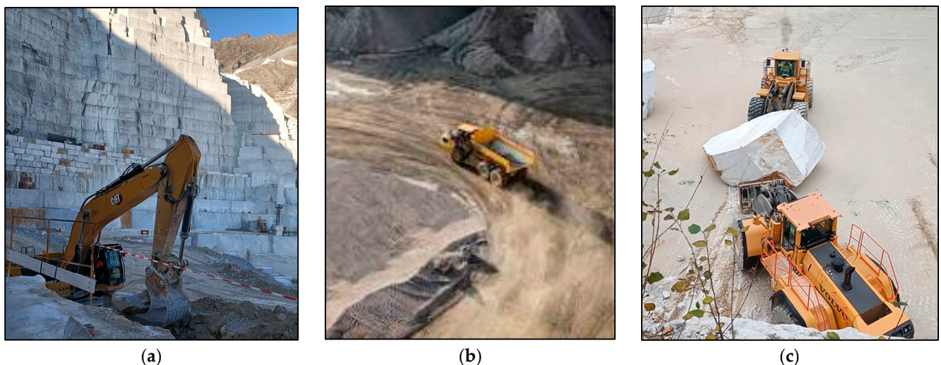
Figure 2. Phases of the standard elementary cycle: (a) Phase A—Excavator clearing waste material to provide access to the block; (b) Phase B—Articulated dumper transports waste; (c) Phase C—Wheel loaders handling and transporting the 20-ton marble block.
