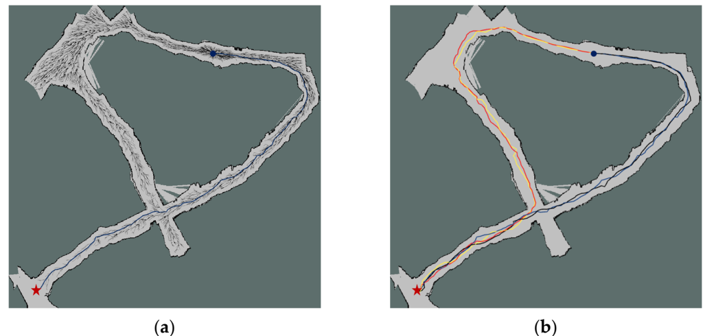
Figure 10. This figure demonstrates the behavior of the RRT* algorithm in narrow tunnels. The start position (blue circle) and goal position (red star) are indicated. (a) Tree expansion during path exploration; (b) trajectory variation across trials due to stochastic behavior described in different colors.
