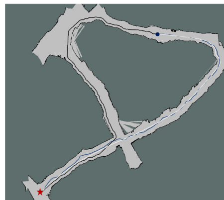
Figure 9. Performance of planners in the simulated Reiche Zeche tunnel. The start position (blue circle) and goal position (red star) are indicated. The trajectories are color-coded as follows: A* (black), Dijkstra's algorithm (white), and RRT* (blue).
