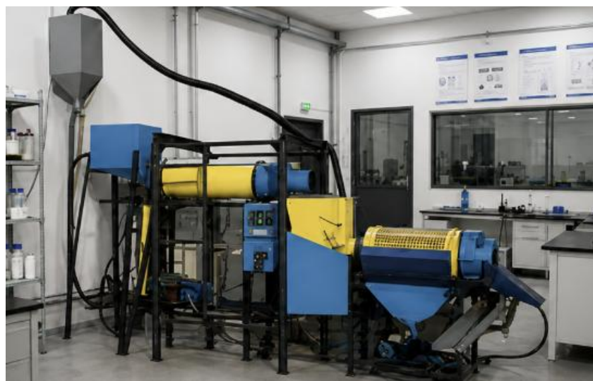
Figure 2. Wet disintegration and classification of bulk ash-slag samples (>100 kg) in a scrubber trommel at RITZ NTK LLP.
