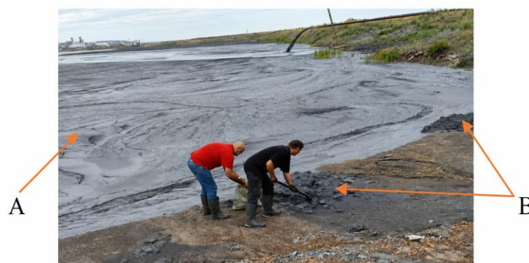
Figure 1. Sampling of ash-slag waste at the aged disposal site: A: general view of the deposit surface; B: sampling locations.
