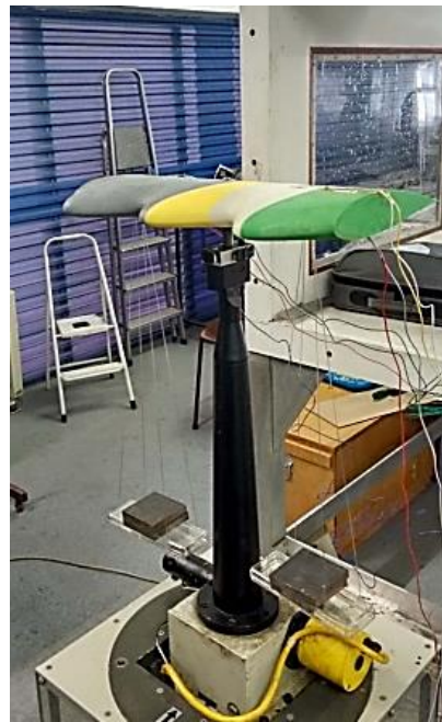
Figure 6. The mounted wing setup and hanging weights.
