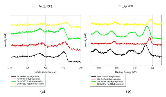
Figure 2. X-ray photoelectron spectroscopy data for both (a) Fe\_2p and (b) Cu\_2p.
