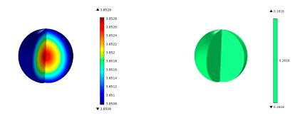
**Figure 6.** Contours of  $C_3H_6$  concentration (mol/m<sup>3</sup>) and formation rate,  $RC_3H_6$  (mol/(m<sup>3</sup> s)), inside a 250 µm radius spherical catalyst pellet (80Fe20Cu/K) at 50 mm from the inlet show very small gradients due to high diffusion coefficients of the gas species at 300 °C and 20 bar total pressure.
