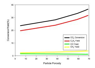
**Figure 7.** Effects of increased particle porosity and decreased bed porosity (with total porosity fixed at 69.7%) on percent  $CO_2$  conversion (black), and percent  $C_3H_6$  (red),  $CH_4$  (yellow), and CO (green) at the reactor outlet as predicted by the model for a fixed 20 g of 80Fe20Cu/K catalyst at 300 °C and 20 bar total pressure.
