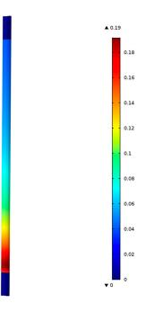
Figure 5. Contours of propene formation rate mol/(m<sup>3</sup> s), RC<sub>3</sub>H<sub>6</sub>, at 300 °C and 20 bar total pressure.
