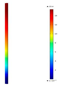
**Figure 4.** Reactor geometry with model-predicted contours of  $C_3H_6$  concentration, mol/m<sup>3</sup>, formed by carbon dioxide hydrogenation in the catalyst bed (20Cu80Fe/K) with bed porosity of 0.51 and particle porosity of 0.38 at 300 °C and 20 bar total pressure at the reactor outlet.
