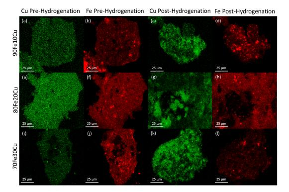
Figure 3. SEM-EDS mapping data where copper is labeled green and iron is labeled blue.
