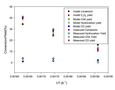
**Figure 10.** Comparison of model predictions with experimental data as functions of inverse temperature for 80Fe20Cu/K catalyst at reactor wall temperatures of 250 °C, 300 °C, and 340 °C and a gas hourly space velocity (GHSV) of  $9.59 \times 10^{-4}$  L/g s.
