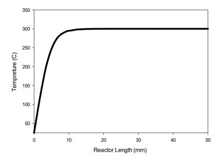
**Figure 9.** Profiles of temperature (°C) along the length (center axis) of the catalyst bed as predicted by the model for 80Fe20Cu/K catalyst at 20 bar total pressure and 300 °C imposed on the reactor wall.
