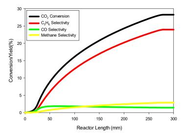
**Figure 8.** Profiles of percent CO<sub>2</sub> conversion (black), and percent C<sub>3</sub>H<sub>6</sub> (red), CH<sub>4</sub> (yellow), and CO (green) yields along the length of the catalyst bed as predicted by the model for 20Cu/80Fe/K catalyst at 300 °C and 20 bar total pressure.
