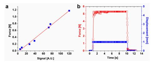
**Figure 6.** Force calibration and validation test of mechanical properties using polydimethylsiloxane (PDMS). (a) The force sensor was calibrated using different scale weights. (b) A stress relaxation test was performed using PDMS of known mechanical properties. A constant displacement (1 mm) was applied to the PDMS, and the reaction force was measured over time. The measured curve shows the typical elastic behavior.
