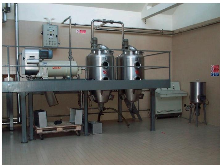
**Figure 6.** Industrial scale ultrasound extraction process (2 × 500 L) as intensification technique for extraction using vegetable oils (Reus—[www.etsreus.com](http://www.etsreus.com)).
