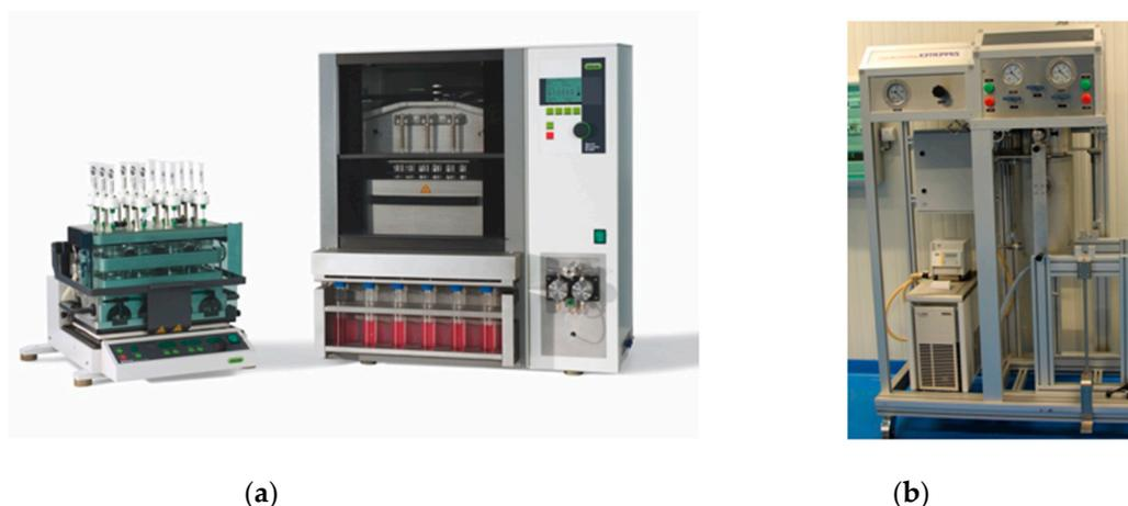
**Figure 2.** Subcritical water extraction system. (a) laboratory scale ([www.buchi.com](http://www.buchi.com)). (b) pilot scale ([www.zippertex.com](http://www.zippertex.com)).
