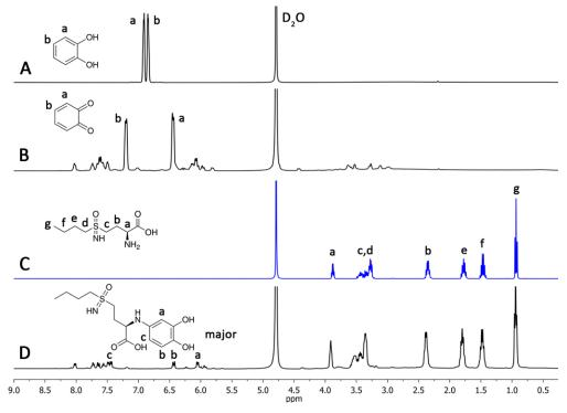
**Figure 4.** <sup>1</sup>H NMR spectra of the L-BSO derivatization reaction followed by NMR. Comparative spectrum of (**A**) catechol, (**B**) o-quinone, (**C**) L-BSO, and (**D**) L-BSO derivative (3). NMR spectra recorded in D<sub>2</sub>O.
