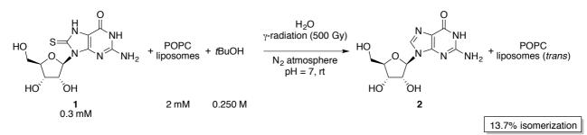
**Figure S8** Reaction of  $e_{aq}^{-}$  with 8-TG in the presence of POPC liposomes.  $\gamma$ -radiolysis of 1 (0.3 mM) in N<sub>2</sub>-purged water at natural pH, containing POPC liposomes (2 mM) and *t*BuOH (0.25 M), at a dose rate of 1.85 Gy min<sup>-1</sup>. The level of isomerization was determined *via* GC analysis
