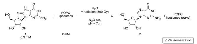
**Figure S9** Reaction of HO<sup>•</sup> with 8-TG in the presence of POPC liposomes.  $\gamma$ -radiolysis of 1 (0.3 mM) in N<sub>2</sub>O-purged water at natural pH, containing POPC liposomes (2 mM), at a dose rate of 1.85 Gy min<sup>-1</sup>. The level of isomerization was determined *via* GC analysis.
