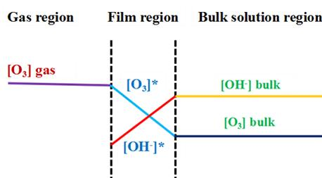
**Figure 4.** The two-film model for ozone oxidation process [47,48].  $[O_3]_{\text{gas}}$ : the concentration of ozone in the gas region;  $[O_3]^*$ : the concentration of ozone in the film region;  $[O_3]_{\text{bulk}}$ : the concentration of ozone in the bulk region;  $[OH]^*$ : the concentration of  $OH^-$  in the film region;  $[OH]_{\text{bulk}}$ : the concentration of  $OH^-$  in the bulk region.
