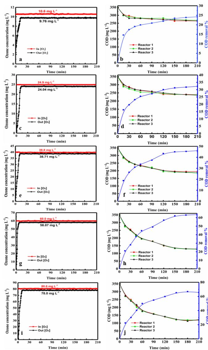
**Figure 1.** Ozone oxidation in the three tandem reactors. (a,c,e,g,i) show the variation in the ozone concentration at the inlet and outlet over time for inlet concentrations of 10.6, 24.9, 39.8, 60.0, and 80.6  $mg \cdot L^{-1}$ , and (b,d,f,h,j) show the change in the COD in each of the three reactors during the ozonation process over time.
