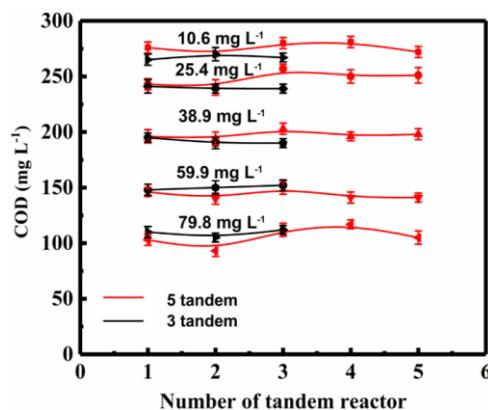
**Figure 6.** The COD at different ozone concentrations at 180 min in the three and five tandem reactors.
