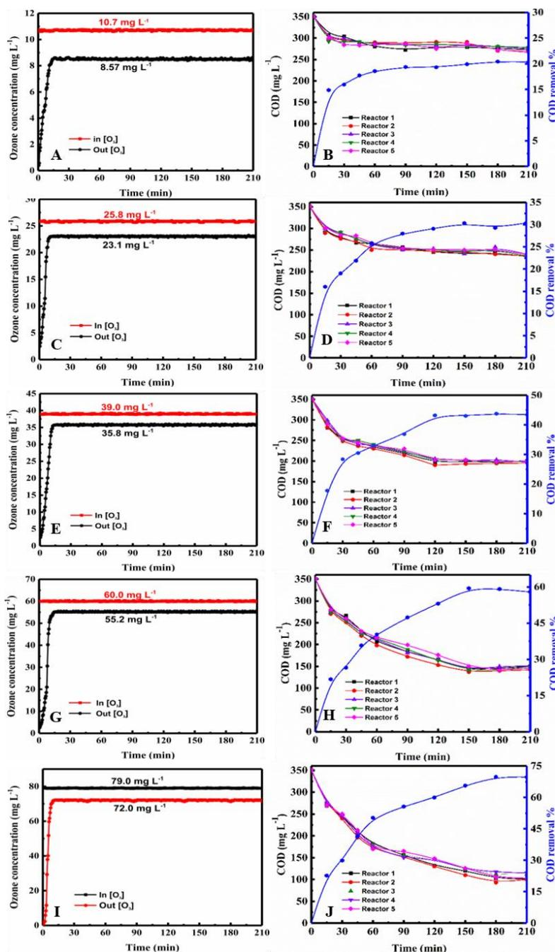
**Figure 2.** Ozone oxidation in the five tandem reactors. (A,C,E,G,I) show the variation in the ozone concentration at the inlet and outlet over time for inlet concentrations of 10.7, 25.8, 39.0, 60.0, and 70.0  $\text{mg}\cdot\text{L}^{-1}$ , and (B,D,F,H,J) show the change in the COD in each of the three reactors during the ozonation process over time.
