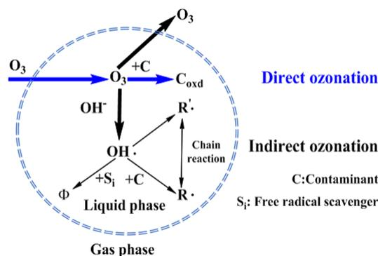
**Figure 5.** The two types of reactions of ozone in aqueous solution [49]. The blue dashed border represents the phase interface between the gas and liquid. According to the two-film model theory, the two dashed blue lines represent the gas-liquid film resistance, as shown in Figure 4. The area outside the circle represents the gas phase, and the ozone dissolves into the liquid phase.
