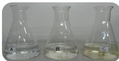
**Figure 9.** Images of biodegradation of the oxidized PML. (A) Raw PML, (B) ozonated PML after 14 days at room temperature, and (C) ozonated PML after 30 days at room temperature. (Experimental conditions: oxidation time: 210 min, oxidation ozone concentration:  $80 \text{ mg}\cdot\text{L}^{-1}$ , room temperature).
