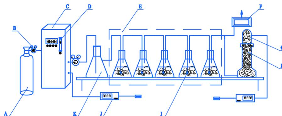
**Figure 10.** Schematic diagram of the three/five-reactor ozone oxidation system. A: oxygen cylinder; B: pressure reducing valve; C: ozone generator; D: rotor flow meter; E: three- or five-reactor system; F: ozone destruction device; G: drying tower; H:  $\text{CaCl}_2$  particles; I: titanium aerator; J: gaseous ozone concentration detector K: buffer flask.
