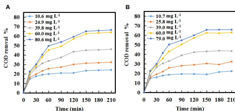
**Figure 3.** Changes in the COD removal % in the second stage of the (A) three tandem reactors and (B) five tandem reactors over time at different ozone concentrations.
