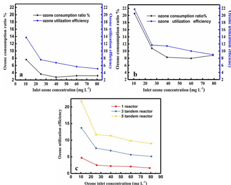
**Figure 8.** Comparison of the ozone consumption ratio and ozone utilization efficiency at different inlet ozone concentrations at 180 min. (a) Three-tandem reactors (b) five-tandem reactors (c) The relationship between the utilization efficiency % and the inlet ozone concentration for the three-tandem reactors and five-tandem reactors at 180 min. The red line in (c) is only one reactor for comparison.
