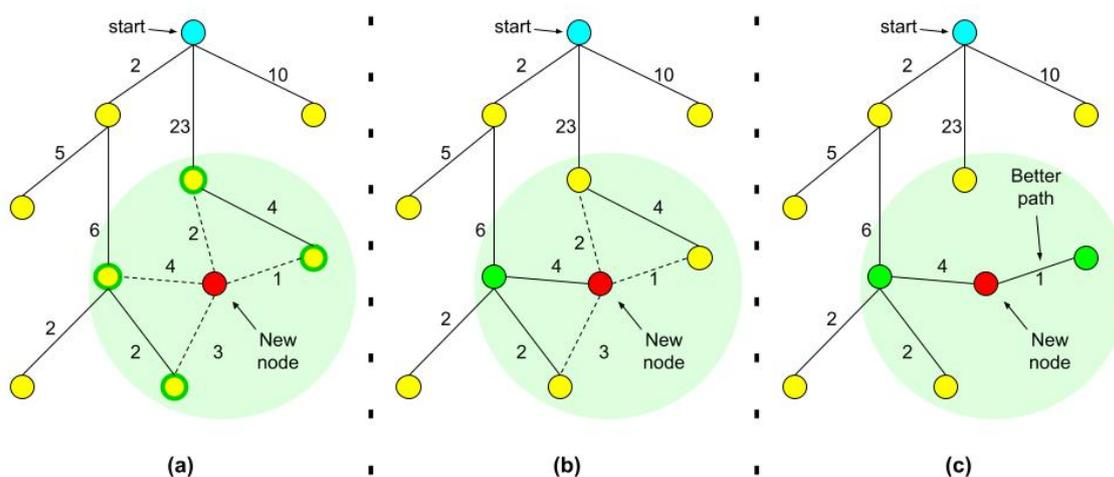
**Figure 1.** Illustration of RRT\* best (least-cost) parent search and the rewiring process. (a) A new node is added to the tree and nearest neighbors are highlighted. (b) The best parent is chosen among nearest neighbors. (c) Costs of rewiring are checked and the tree is rewired.
